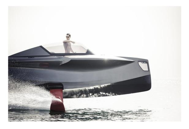
AGAMECHANGERSUPERYACHTTOYFor ease of maintenance, the retractable hydrofoils and propellers are lifted and positioned outof the water when not in use, which also reduces the yacht's height for storage and is particularlyconvenient for stowage in superyacht garages.
